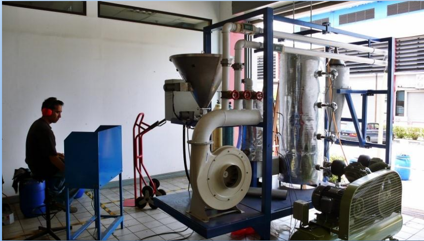
Two-stage combustor to simulate real boiler
