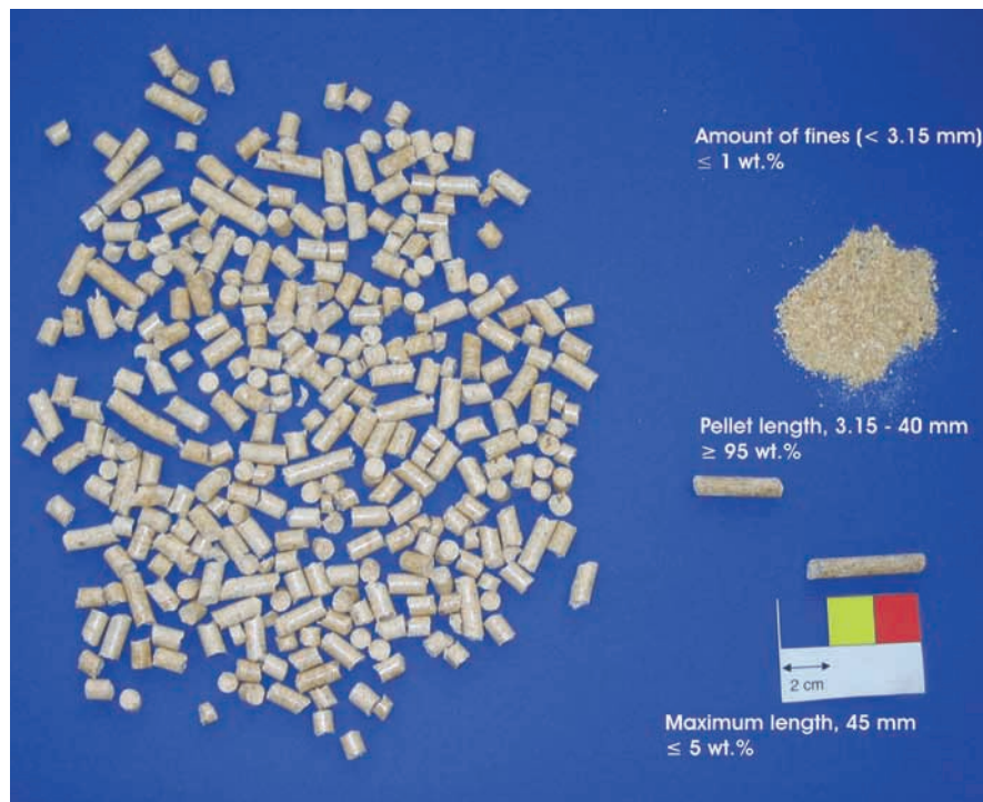
Figure 1: Wood pellet classification according to EN 14961-2. [27]
