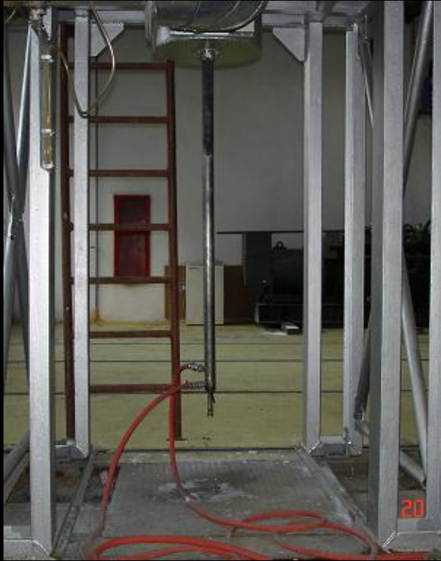
Collecting ash depozits on ceramic probes and water cooled lance
