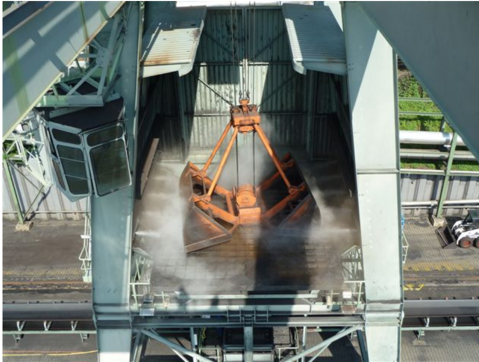
Unloading with water dispersion system in operation (top view)
