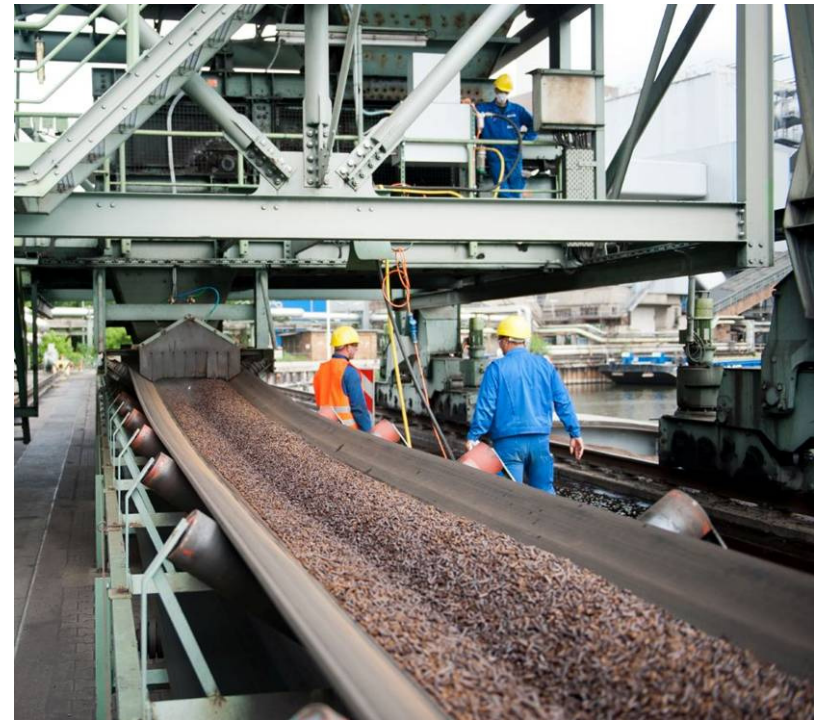
Transfer point from ship unloader to conveyor belt with water dispersion system in operation
