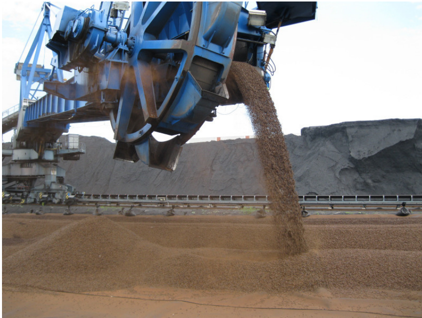
Stacker/Reclaimer in operation
