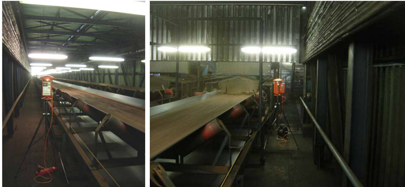
Airborne dust measurements within at a.) conveyer belt and b) transfer point at tower
