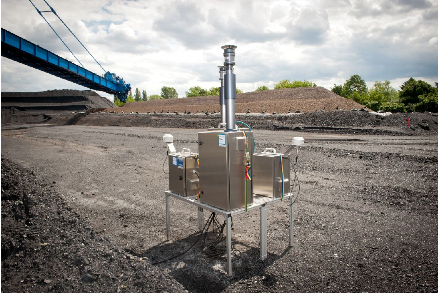
PM 10 and PM 2,5 fine dust measurement device at Reuter West coal yard
