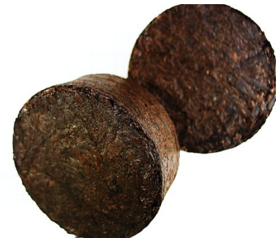
Test briquetts from ACB material source: TU-Freiberg
